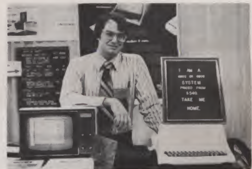
Steve Alcorn of MicroDaSys (Box 36051, Los Angeles CA 90036) says that his MicroDaSys computer is now available with either a 6800 or a 6809 chip. The TV monitor shows a dump of memory done with the MicroDaSys monitor program—but, unlike other monitors, the user can modify any byte shown on screen by simply writing over the byte's current value.
